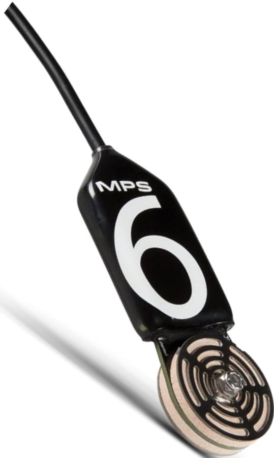
*The MPS-6 is a matrix water potential sensor that provides long term, maintenance-free soil water potential and temperature readings at any depth without sensitivity to salts. The range of the MPS-6 goes from field capacity to air dry. Lab and field tests indicate that it can make accurate measurements at water potentials at least as dry as permanent wilting point.*
